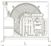
The standard equipment of E-AU units includes an air-cooled condenser with copper pipes and new design aluminium fins, high efficiency electric motor-fans equipped with safety grill, liquid receiver with safety valve and anti-vibration damper on discharge piping (when included), gas and liquid piping, steel frame
