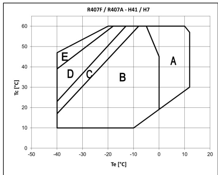
The application envelope changes depending on the compressor model and is available for every model and for every refrigerant in the DORIN web software
